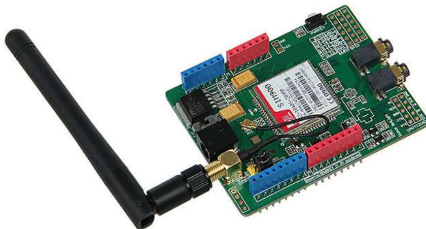
სურ 8.2. SIMCOM SIM900 Module Quad Band Wireless GSM/GPRS Shield
