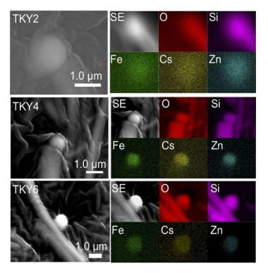
Image above: Secondary electron images from Utsunomiya et al. 2019, of CsMPs discovered in atmospheric particles trapped on a Tokyo air filter from March 15, 2011, with major constituent elements displayed.
