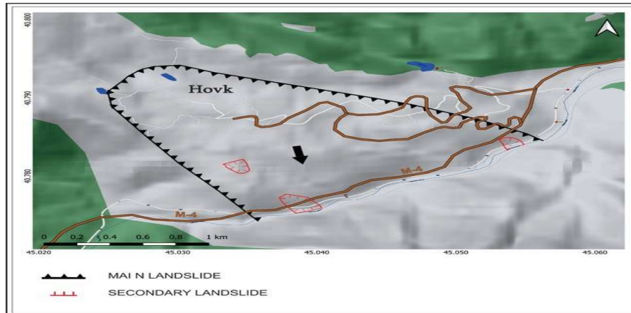
Fig. 1. Structure of the Hovq Community landslide, black lines outline the general area of the landslide (main landslide body), and red lines contour the secondary landslides that have developed this year
