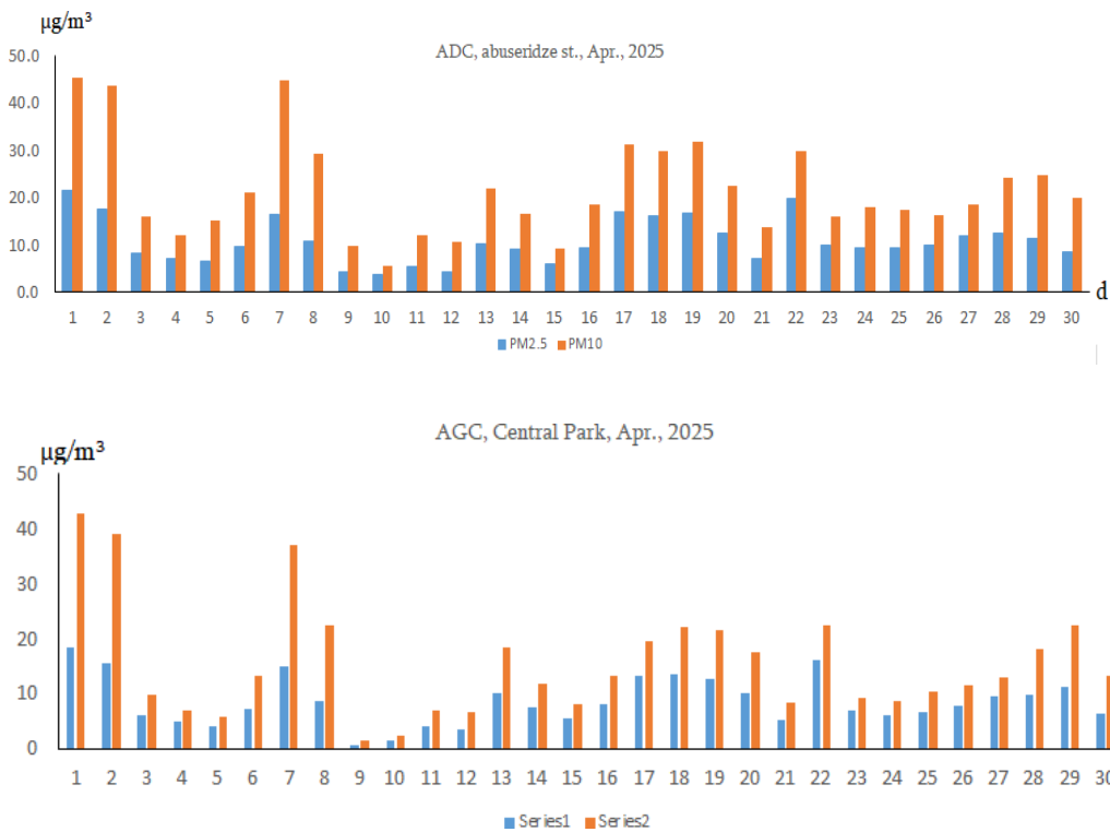
Fig. 4. ADC of PM2.5 and PM10 in April at the observation points T. Abuseridze and Central Park.
